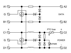
voltage on the power supply line. To reset the resettable fuse, the circuit must be switched off and let the fuse cool down. Unlike a standard fuse, resettable fuses do not have to be changed, which can reduce the service interventions or make the service faster.
